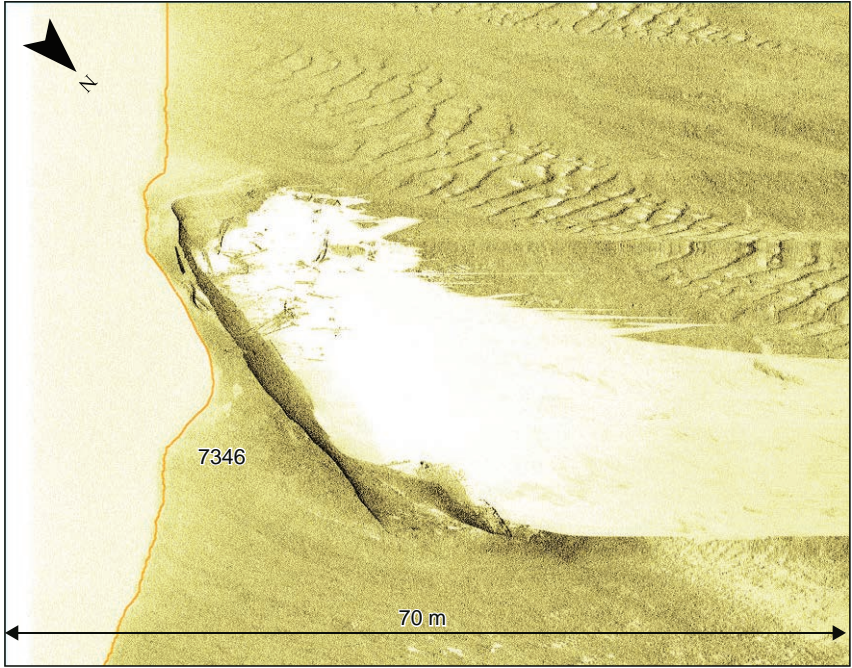
Sidescan sonar waterfall image of wreck 7346 , measuring 70 m range per channel
